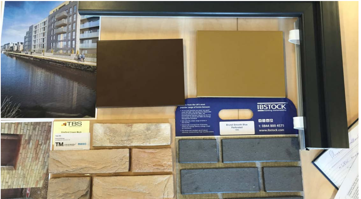
Barchester Street: the impact of different mortar colours, bonds and brick patterns being reviewed for works
