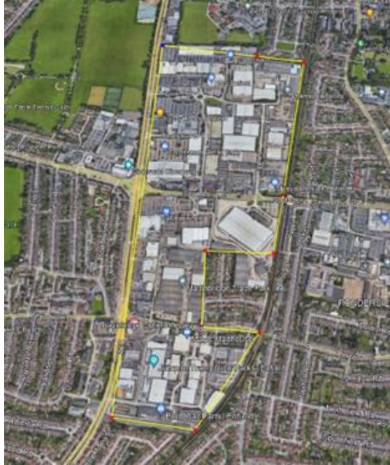
Figure E.39: Potential area to implement SuDS options for disconnection at Colosseum retail park
