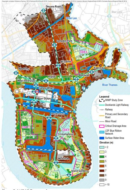
Figure 3-4 LiDAR Topography (Appendix A Figure 3)
