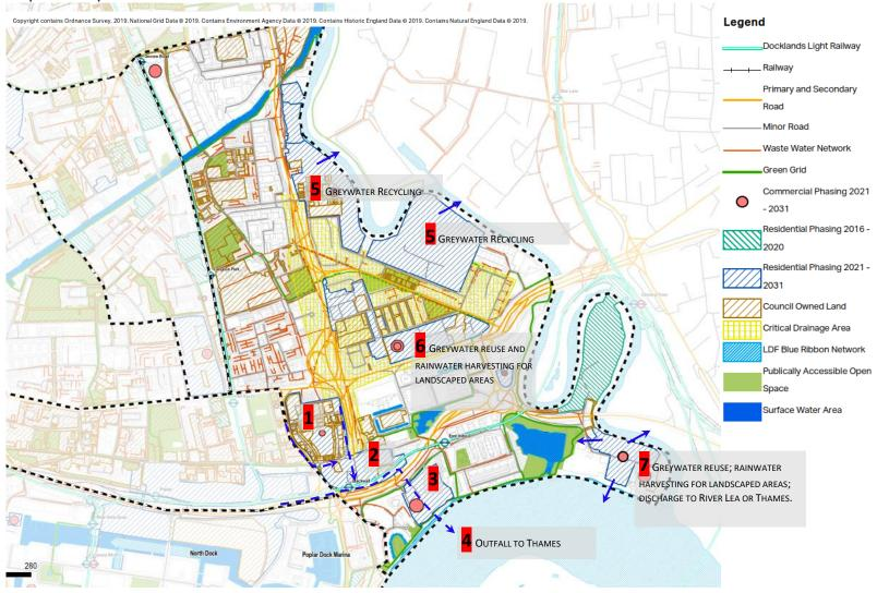
Figure 6-18 Schematic of Options for Zone 6A AAP Core Area
