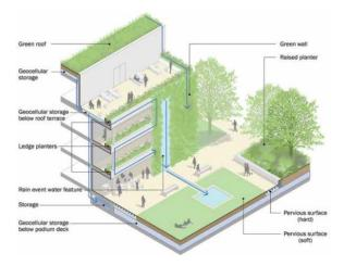
Figure 6-14 Example of multi-functional use of elevated surfaces. SuDS Manual C753.
