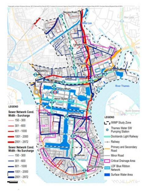
Figure 3-9 Thames Water Sewer Network Capacity Assessment (Appendix A Figure 9)
