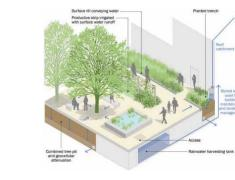
Figure 6-24 Example of rainwater harvesting system combined with surface water attenuation. SuDS Manual 753
