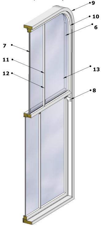
Typical timber sash window components
