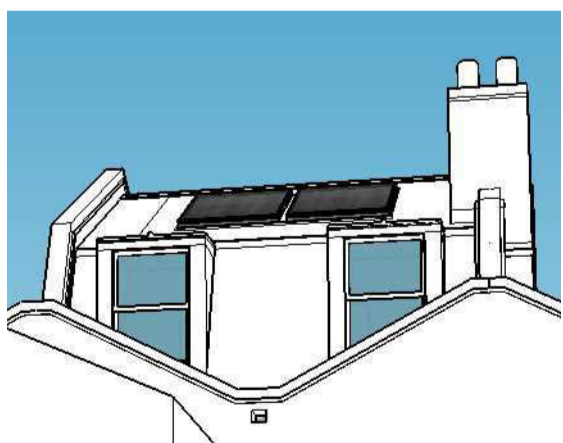
In-line panels sit flush with the roof and look more like rooflights
