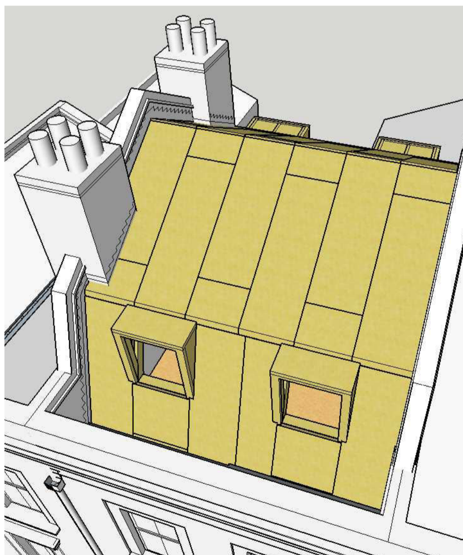
Fix racking boards over rafters. These can have insulation properties to reduce cold-bridging, heat loss and heat gain. Additional insulation will be required to meet building regulations
