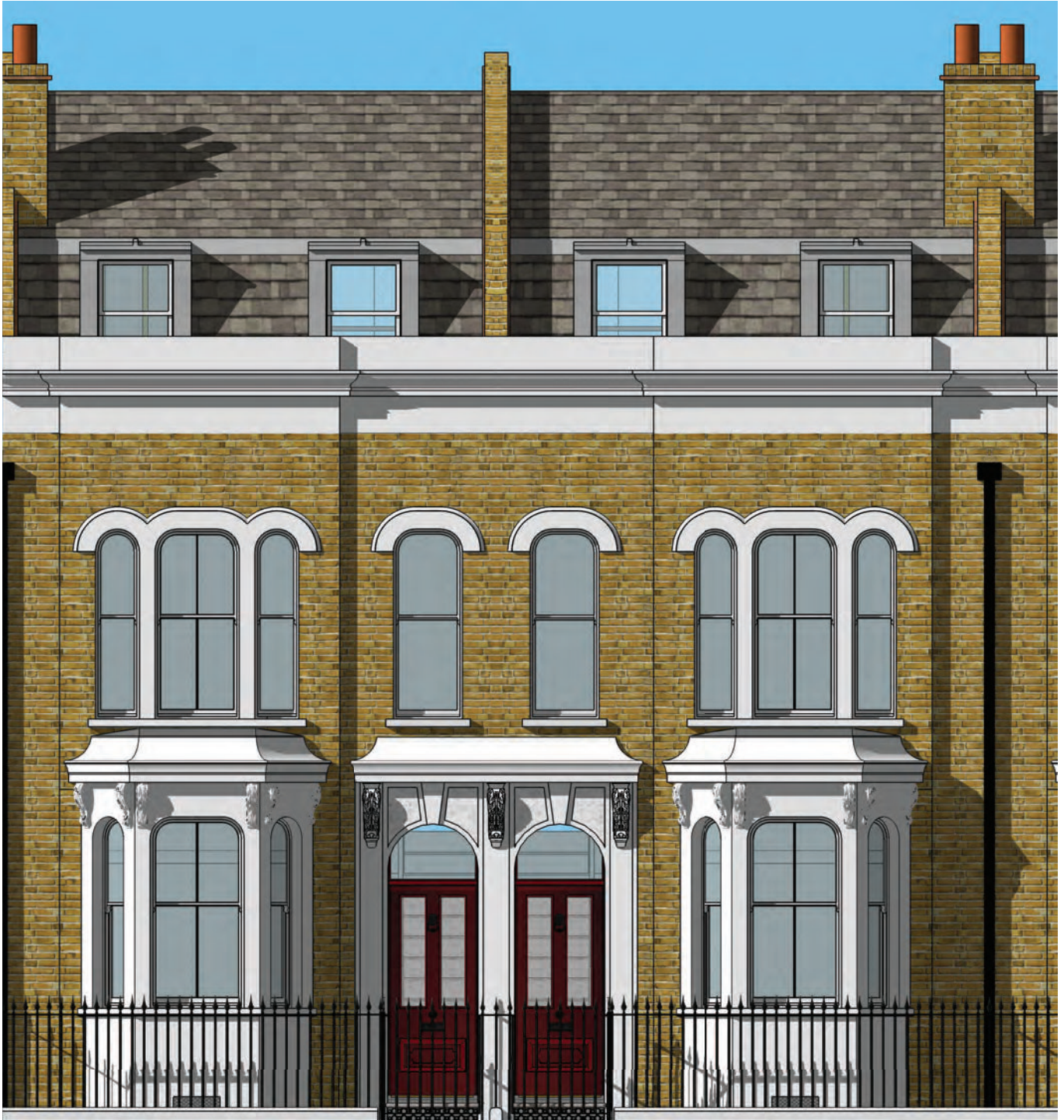
Prototype elevation of typical properties in Medway Conservation area with roof extensions and architectural features reinstated
