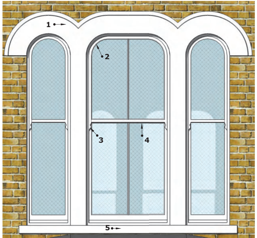
Typical timber sash windows in Medway Conservation Area. It is important to retain the curved head. The numbers are explained in the text
