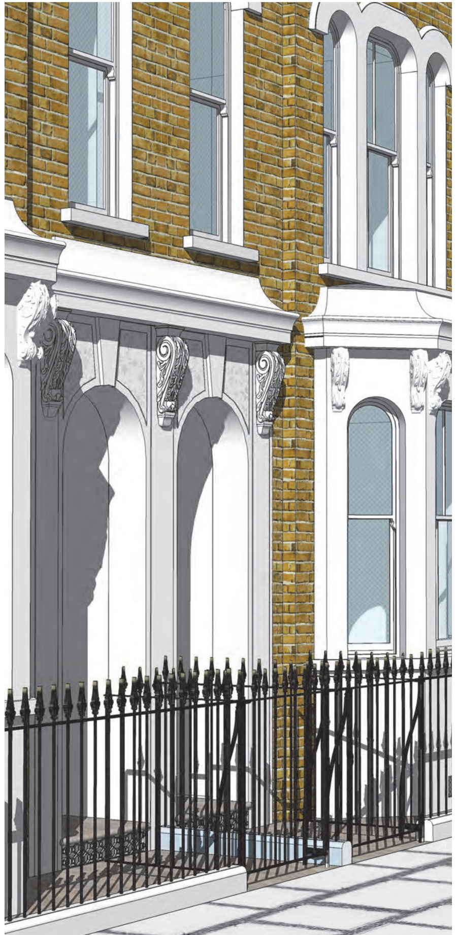
Prototype model drawing of acceptable railings, with 20mm bars caulked into the plinth
